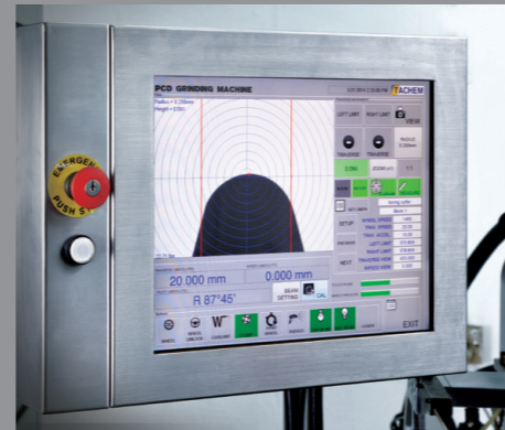
17" heavy duty industrial touch screen monitor. In process dimensional measurement.
